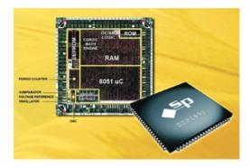
Available in 4.3 x 4.3-mm bare die and a variety of surface-mount packages, the chip includes two hardware math engines, a software floating-point engine for high-order output linearization and temperature compensation, a band-gap reference, an SPI/I<sup>2</sup>C serial interface, an RC oscillator, and an EEPROM for factory calibration coefficients and user settings. An evaluation kit is available. (From \$3.65 ea/1,000—available now.)
